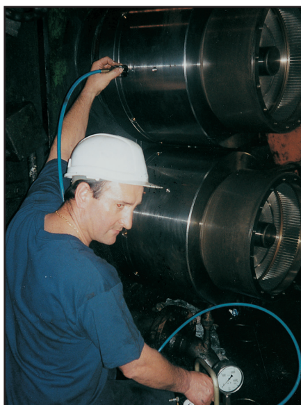
Pumping oil into a spindle with Safeset®
