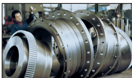
Main Drive Gear Coupling
